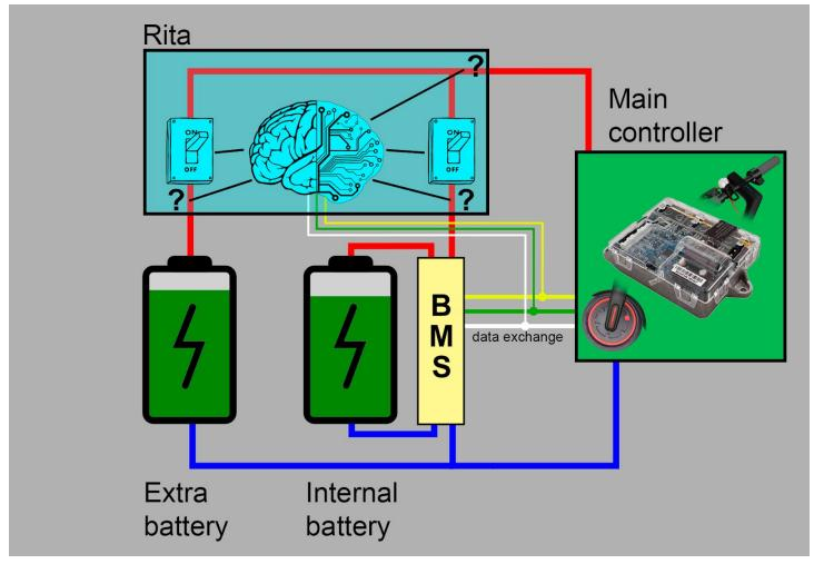
Rita analyzes the voltages of the internal and additional external batteries, and switches their positive power leads so that the charge does not flow from one battery to another, at the same time keeps the ability for the controller to consume current from both batteries and recover energy back when braking.
