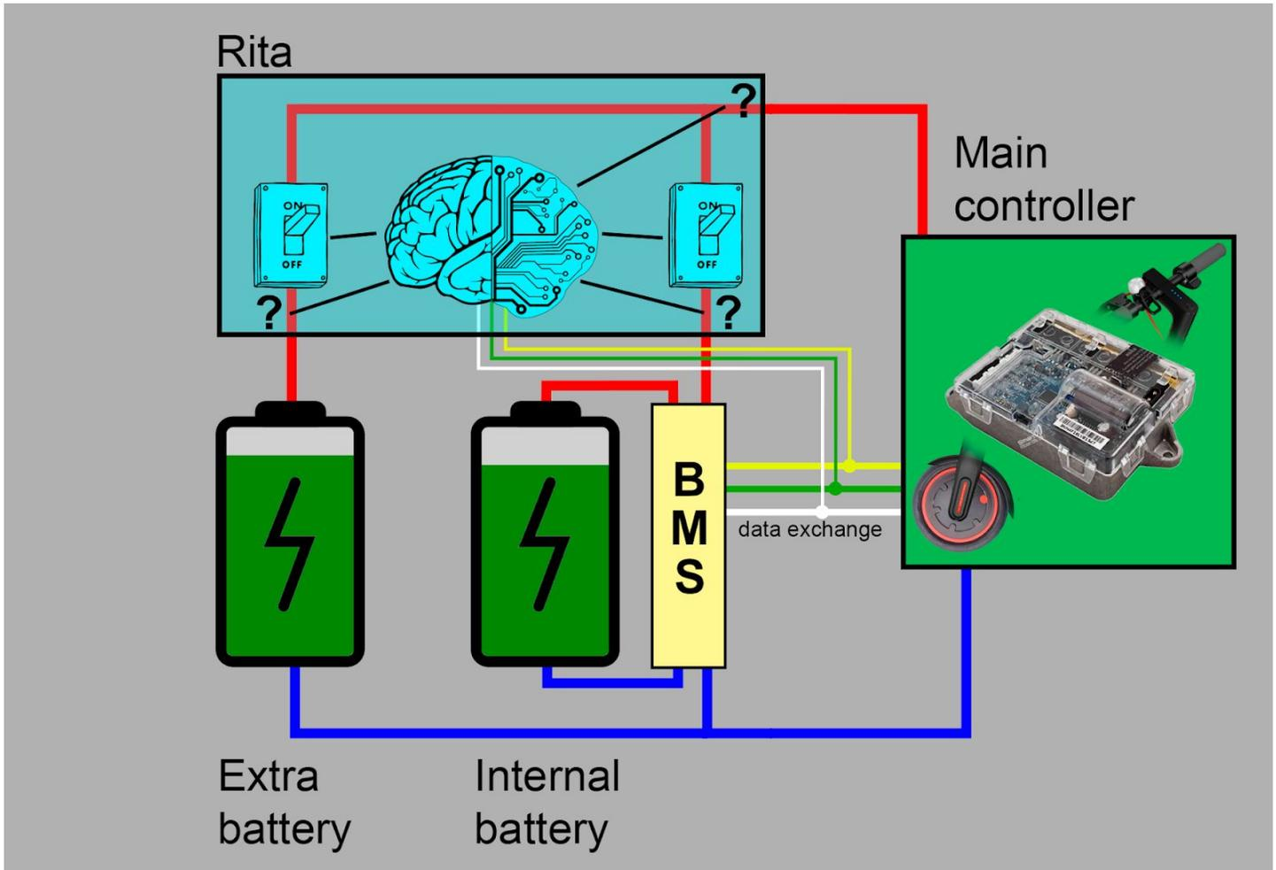
Rita analyzes the voltages of the internal and additional external batteries, and switches their positive power leads so that the charge does not flow from one battery to another, at the same time keeps the ability for the controller to consume current from both batteries and recover energy back when braking.
